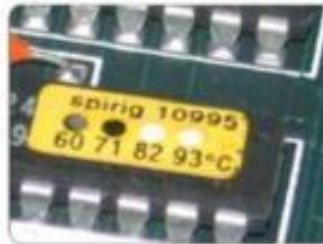
CalibrCheck with 7 temperature levels. CalibrCheck's are also available with other temperature values and arrangements.
