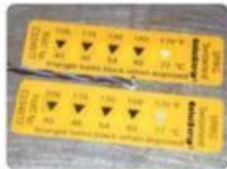
CalibrBright with 7 temperature levels. Also 6 levels (not shown here) available. Also 6°C are available for TTC water washed.
