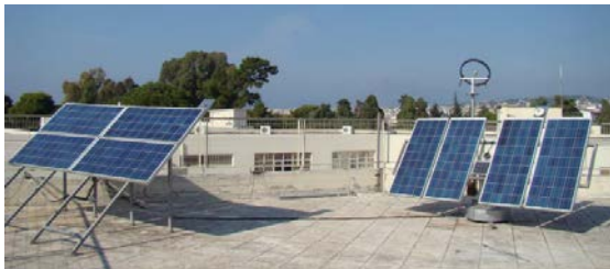
Picture 2-7 A sun-tracking PV system vs a fixed inclination one. 4 PV panels pc-Si of 122 Wp each are mounted on both frames, at Renewable Energy Sources Laboratory at technological educational institute of Western Greece, Patra.
