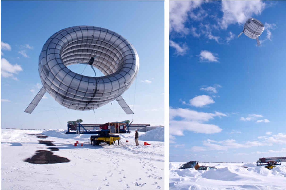
Picture 2-3 Airborne wind turbine by Altaeros Energies company. A viable clean energy option for remote villages and military sites.
