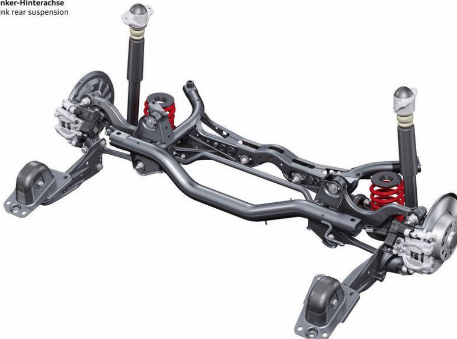
Audi A3 Sportback Mehrlenker-Hinterachse Multi-link rear suspension
