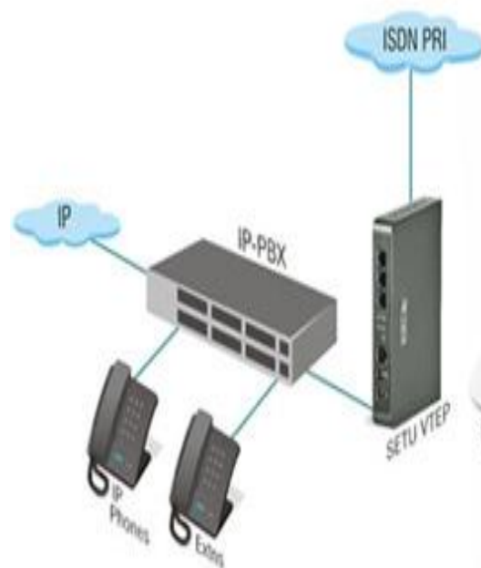
VoIP Access for ISDN PBX
